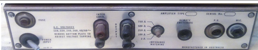
Steanes PA. Circa mid 1950. Typical Steanes/ Philips rear connections with switched speaker impedances. Just before Philips took over formally.
