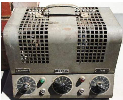
Circa 1952; unbranded; uncommon mic sockets on front; no mains fuse or switch.
