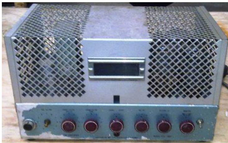
AWA 70W PA827 – retrofitted front panel socket and power switch.
