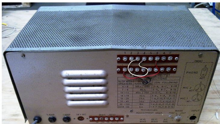
Rear of AWA PA1001; multiple speaker screw terminals; bass cut switch. Inputs on side panel.
