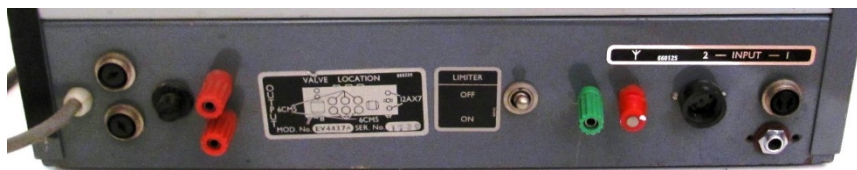
Typical looking late Philips PA and rear connections. Layout & input labels. 100V line output only.
