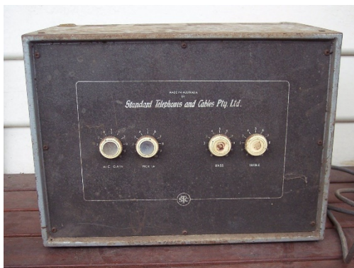
STC used a large upright PA layout, along with Ferguson transformers for a range of amps from 20W to 60W.
